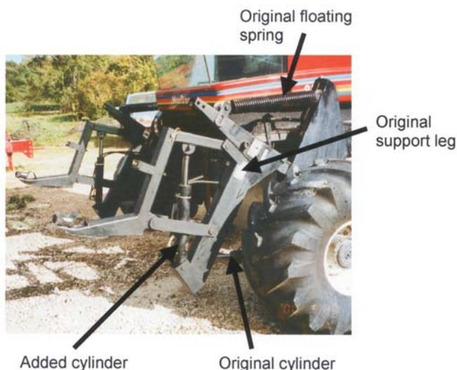
**Fig. 4. The new combined header-lifting mechanism.**
